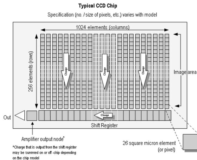
The **Shift Register** runs below and parallel to the light collecting rows. It has the same number of pixels as a light-collecting row, but is itself masked, so that no light can fall on it. When light falls on an element, electrons (photoelectrons) are produced and (in normal operation), these electrons are confined to their respective elements. Thus, if an image (or any light pattern) is projected on to the array, a corresponding charge pattern will be produced.
