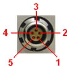
Figure 11: I²C connection (facing in) with pinouts
