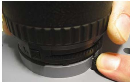
Press the catch down, screw the lens in carefully counter-clockwise and it will then lock into position
