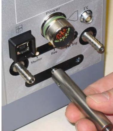
Figure 8: Fitting a mounting post
